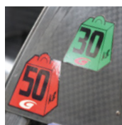
The decal on the side of the car shows how much weight is imposed to the car.
