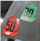
The decal on the side of the car shows how much weight is imposed to the car.
